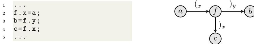
Fig. 1: Modeling program behavior with language graph reachability. Parentheses are used to match field accesses on the composite object  $f$ . The balanced path  $a \xrightarrow{(x)} f \xrightarrow{)x} c$  captures the fact that  $a$  flows into  $c$ . On the other hand, as the path  $a \xrightarrow{(x)} f \xrightarrow{)y} b$  is imbalanced, it does not witness the flow of  $a$  into  $b$ .
