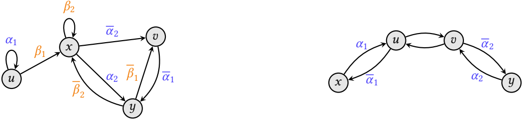
Fig. 2. (Left): An interleaved Dyck graph. We have u \stackrel{\mathcal{D}_1 \odot \mathcal{D}_1}{\rightsquigarrow} v , via the path u \xrightarrow{\alpha_1} u \xrightarrow{\beta_1} x \xrightarrow{\beta_2} x \xrightarrow{\alpha_2} y \xrightarrow{\beta_2} x \xrightarrow{\alpha_2} y \xrightarrow{\beta_2} v . (Right): A bidirected Dyck graph. We omit the \epsilon label from the edges.
