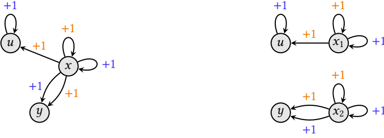
Fig. 9. (Left): A bidirected, interleaved Dyck graph G with a doubly-self-looped node x . (Right): The two connected components on which we perform \mathcal{D}_1 \odot \mathcal{D}_1 reachability separately in order to infer whether x is reachable from any other node.
