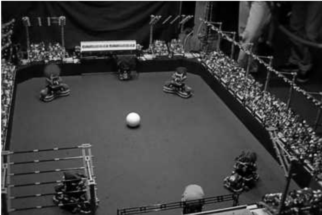
Figure 3. The LEGO robot soccer set-up that was used during RoboCup'98. There are two field players and a goalkeeper on each team. © H. H. Lund, 1998.
