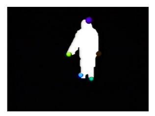
Figure 2: Simple vision routines extract figure from background and label salient points of contour.
