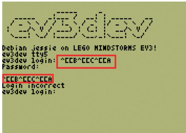
Figure A.16: When a program is running on the EV3 button events are not fully intercepted by the running program, but are also executed in the terminal. This results in input showing up on the EV3 screen, as marked by the red boxes, when the buttons on the EV3 are pushed.
