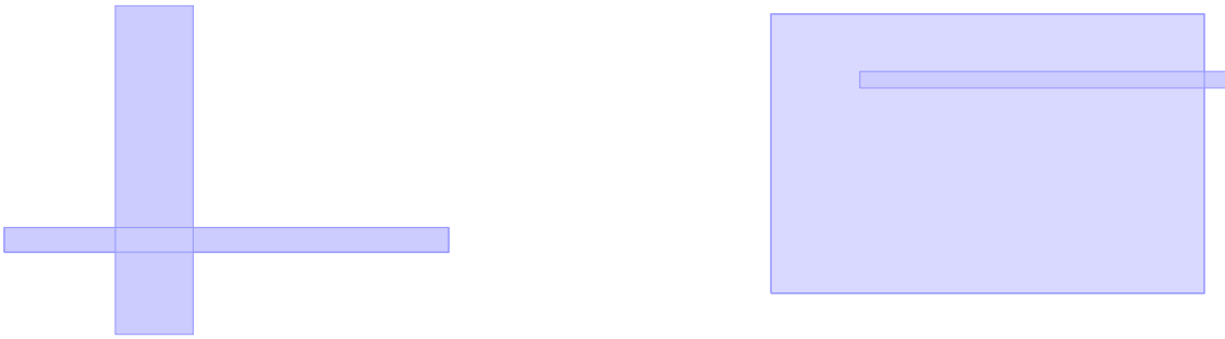
Figure 2: When boxes differ a lot in side length for at least one of their dimensions (in this case, the y -axis), their intersection is small compared to their union.
