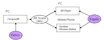
Figure 1. The structure of the mobile AR authoring system.
