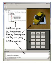
Figure 2. The ComposAR-Mobile Interface.
