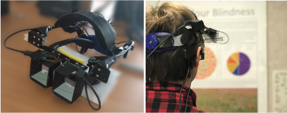
Fig. 16. Left: Our portable prototype based on the Lumus DK-52 modified to increase stability. Right: Participant wearing the prototype in front of the poster.
