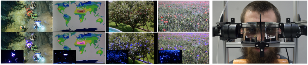
Fig. 1. Examples demonstrating the results from using Computational Glasses to create a spectral wave-length shift for CVD. Top: Pictures presented in front of a user wearing our prototype. Bottom: The pictures when viewed using a compensation technique, insets demonstrate what is displayed on the glasses. Note that these are exaggerated compensations for paper clarity. Right: The large, stable stereoscopic prototype used for controlled user studies. All images were captured through this system and are not simulated. We also demonstrate the development of smaller portable versions.
