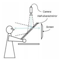
Figure 4. Schematic of half-silvered mirror approach
