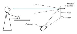
Figure 2. Schematic of hole in screen approach
