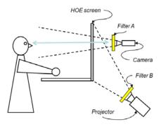
Figure 7. Schematic of "i2i" (HOE and filters) approach
