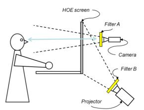
Figure 2. Schematic of "i2i" approach. A Holographic Optical Element (HOE) is used to separate the camera view from the projected video conferencing image. Additional polarization filters are added in the light path.
