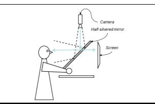
Figure 6 Schematic of half-silvered mirror approach as described by Kannes (1990, 1995).
