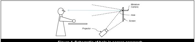
Figure 4. Schematic of hole in screen approach
