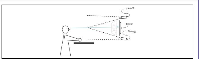
Figure 7. Schematic of 2D video interpolation approach. In some prototype systems a computer-vision approach is used to synthesize/interpolate the views of multiple cameras around the screen to compute an image from a virtual camera place in front of the user's eyes, which is then transmitted to the conferencing partner
