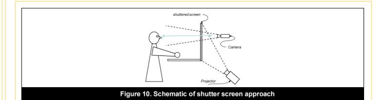
Between update cycles of the system a black projection image is rendered and a camera image is captured. During that period of time the screen is transparent because a shutter glass is used and triggered to transparent mode synchronously. Hartkop (2007) placed cameras behind an OLED screen synchronizing the video camera(s) with the OLEDs illumination levels for the same purpose.
