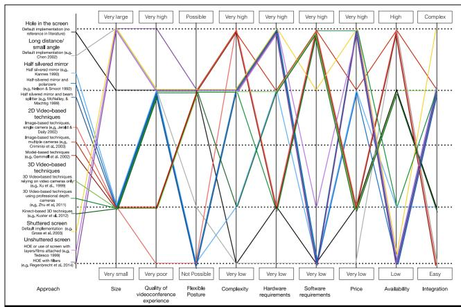
Figure 11. Parallel line plot visualising the main approaches for eye-to-eye videoconferencing and their performance according to our criteria's. As one can see there are a wide variety of different approaches with different strengths. However, all existing approaches have also major drawbacks. Usually either the hardware or the software requirements are very high but still don't guarantee perfect quality.
