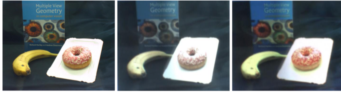
Fig. 12. Incorrect colour reproduction in OST-HMDs. (Left) A physical scene captured by a user-perspective camera representing the intended target colours. (Middle) Rendering the captured image with an OST-HMD in front of a fully black background produces a different result. (Right) The result of the correction method proposed by Itoh et al. produces a result that is more consistent with the captured physical appearance [58]
