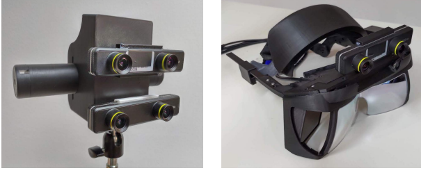
Figure 8: System configurations. The setup used for evaluating EPR techniques and their impact in view management for OST HMDs. (Left) We use the Stereo ZED Mini to capture I_{H,RGBD} representing a typical camera of an OST HMD. A second Stereo ZED Mini placed at the position of the user’s eyes represents the user’s view and captures ground truth images I_{E_i} later used for comparison against the synthesized views I_{E_i} . (Right) The setup with the Project North Star OST HMD and one of the Stereo ZEDs attached directly to the HMD. The HMD was used in the second user study by study participants. When capturing views through the display, the device was attached to the capturing rig on the left where the HMD camera replaced one of the capturing rig.
