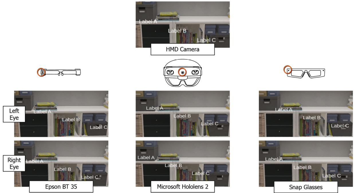
Figure 2: Illustrating the mismatch between HMD camera and user’s eyes. We measured the offset between the built-in HMD camera and the user’s eye for various commercial AR HMDs and created renderings for a Unity scene illustrating this offset for left and right eye of the user. Labels are placed at 70cm from the HMD, the scene is approximately 2m from the HMD. The background behind the labels changes with each device and eye perspective compared to the HMD camera view. Displacements depend on the location of the HMD camera relative to the user’s eyes. Note that, due to the stereo perception of the labels, the label background is different for left and right eye, which can lead to perceptual issues when reading labels.
