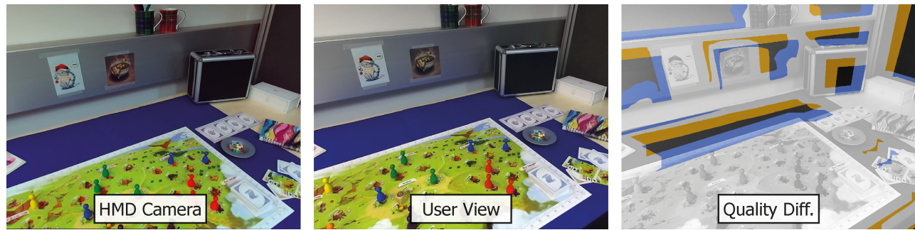
Figure 3: Optimization criteria utilizing incorrect scene information. (Left) The HMD camera view and the (Center) user's real view capture a real-world scene from different perspectives. Therefore, optimization algorithms like view management rely on incorrect scene information when utilizing the HMD camera's view to optimize content for the user's view. (Right) Blue, yellow and white overlays illustrate the results of an optimization criterion utilizing HMD camera information, overlaid over the user's view. Blue indicates pixels that are incorrectly classified as valid regions in the HMD camera view. Yellow indicates pixels that are valid in the user's view, but have not been detected in the HMD view. White indicates results that are correctly classified despite the offset, due to visual similarity between HMD camera view and the user's view in the respective area.
