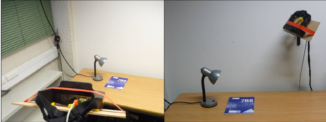
Figure 6. OST HMD positioned further from the scene so it is able to virtualize the entire scene (left), and then the HMD positioned close enough to the scene so the interaction component is able to be visualized (right).
