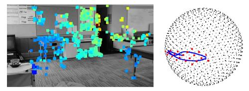
Figure 3: Example output of our system. Left: tracked features overlaid with the current input frame. Right: Tracked poses (blue) alongside, occupied (red), and unoccupied (black) keyframe anchor points.
