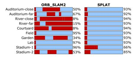
Figure 7: Tracking timelines of ORB\_SLAM2 compared to our Spherical SLAM system across ten video sequences at 540p video resolution. Blue represents a successfully tracked frame, red represents an untracked frame. We show the percentage of successfully tracked frames (metric B) alongside each sequence.
