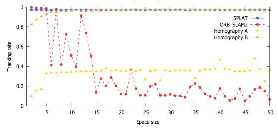
Figure 6: Tracking rate of our spherical tracker (blue), ORB\_SLAM2 (red), and a homography-based tracker (with two metrics: yellow and orange) on our synthetic video sequences with different 3D sphere radii.
