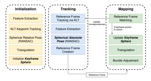
Figure 4: High level overview of our tracking and mapping system. The first component handles initializing a 3D map, and the Keyframe Sphere before handing off to the tracking component. The tracking component tracks keypoints from the last reference frame, and creates new reference frames when required by the Keyframe Sphere. The mapping thread updates the 3D-to-2D matches of the latest reference frame asynchronously, triangulates new points, and updates the Keyframe Sphere.
