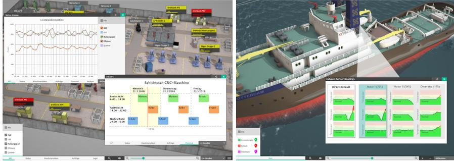
**Fig. 6.** Examples of visual data analysis use cases with *Plant@Hand*: factory visualization (left) and ship condition analysis (right).
