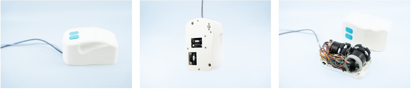
Figure 1: The CASTOR mouse with its two omni-wheels protruding from the bottom and the BLDC motors inside the shell.
