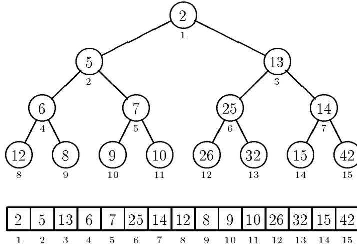
Figure 1: A binary heap of size 15 and its implicit representation.
