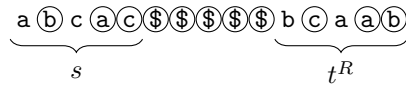
■ Figure 2 The reduction of \text{LCS}(s, t) to \text{LPS}(s^n t^R) . The circled symbols are an LPS of s^n t^R , and the circled symbols of s are the corresponding LCS of s and t .
