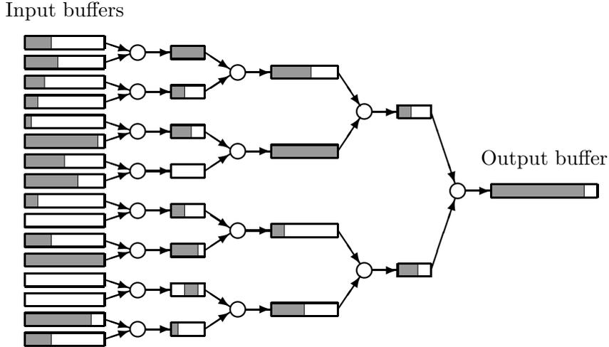
Figure 2: A 16-merger consisting of 15 binary mergers. Shaded regions are the occupied parts of the buffers.
