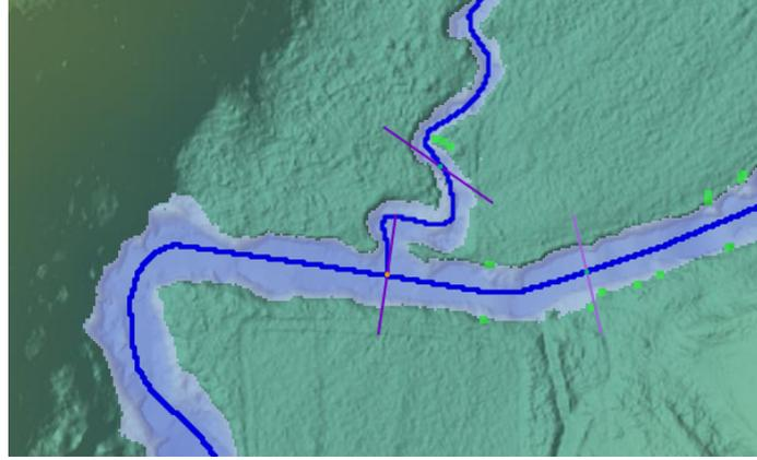
Figure 5.9: A 2D channel from a 1D network using Manning's equation. The 1D network is given in dark blue and cross sections in purple. The figure is generated using SCALGO software [91].
