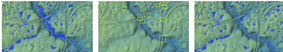
(a) Flash flood simulation without hydrological corrections. (b) Hydrological corrections. (c) Flash flood simulation with hydrological corrections.
