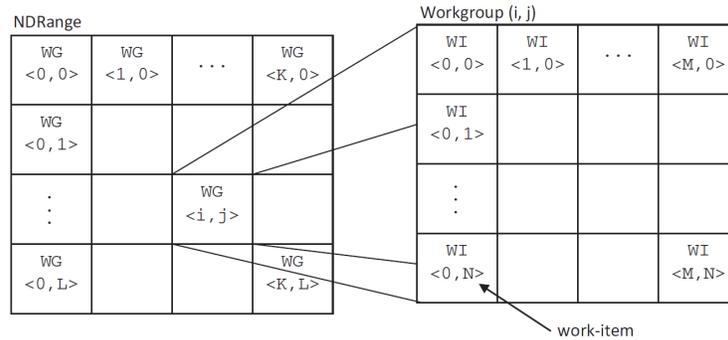
Figure 7: An example of a two-dimensional NDRange of work items in their respective workgroups. Source: "*Heterogeneous Computing with OpenCL*" [8].
