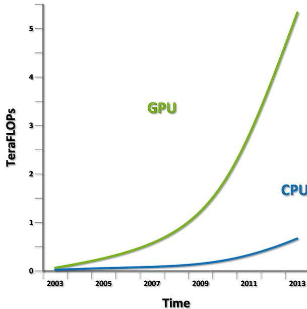
Figure 5: A graph that shows the development in raw single-precision compute performance in GPUs and CPUs. Source: Nvidia.
