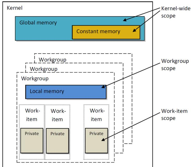
Figure 8: The OpenCL memory hierarchy. Source: "*Heterogeneous Computing with OpenCL*" [8].
