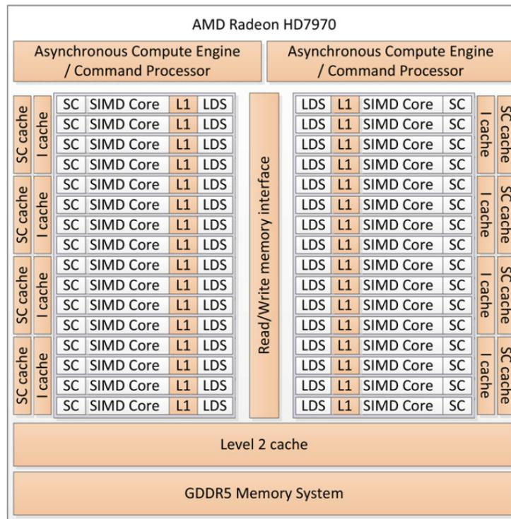
Figure 6: A block diagram of AMD's Tahiti architecture. Source: "*Heterogeneous Computing with OpenCL*" [8].
