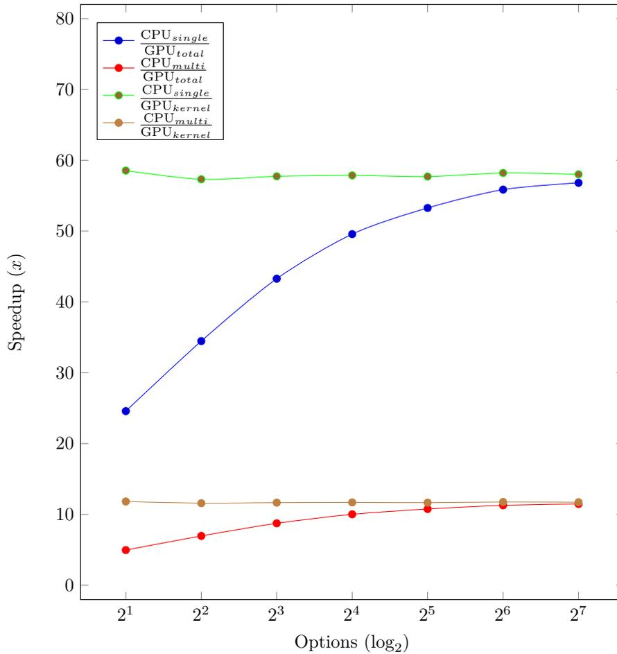
Figure 20: Plot showing the relative performances of  $\text{GPU}_{total}$  and  $\text{GPU}_{kernel}$  versus the CPU performances for single-thread and multi-threaded versions.
