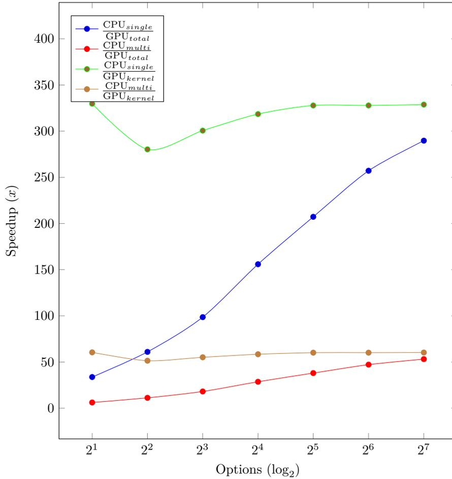
Figure 17: Plot showing the relative performances of  $\text{GPU}_{total}$ ,  $\text{GPU}_{kernel}$  versus the CPU performances for single-thread and multi-threaded.
