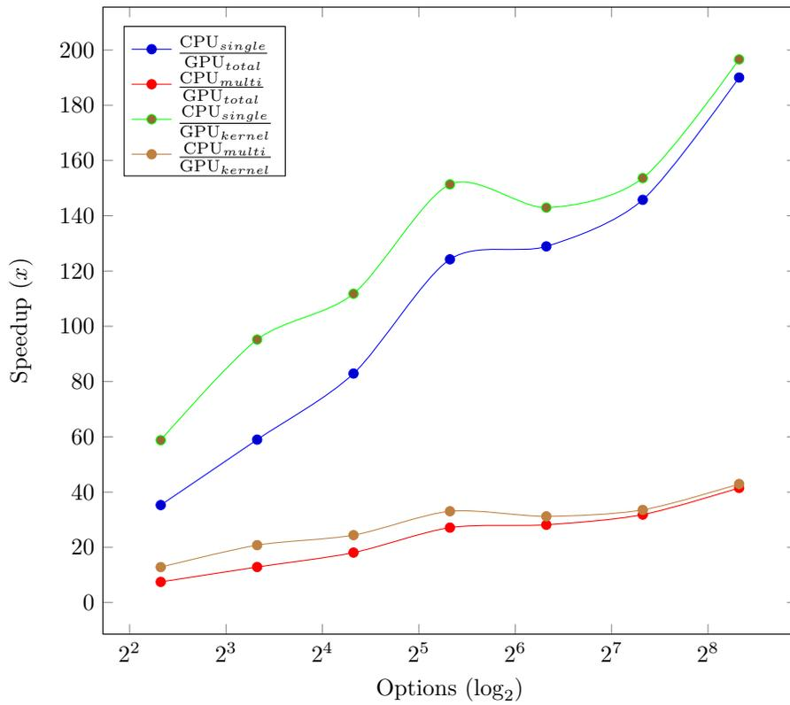
Figure 14: Plot showing the relative performances of GPU<sub>total</sub>, GPU<sub>kernel</sub> versus the CPU performance for single-thread and multi-threaded.
