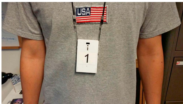
Fig. 10. The wearable sociometric badge used in the design session. The badge, developed by Sociometric Solutions (now Humanyze: http://humanyze.com ), measures individual biometric data including speech events and body movement, as well as social interactional data such as face-to-face interactions, conversational overlaps, turn-taking, and proximal connections.
