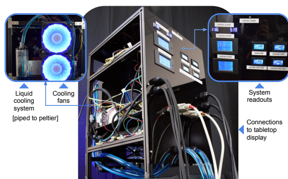
Figure 2: The viScent 2.0 control tower.
