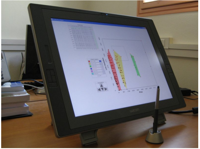
Fig. 8: Wacom CintiQ 21UX graphical tablet used for the visual exploration scenario, here shown running our prototype implementation.
