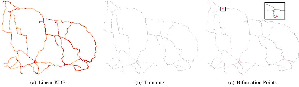
Figure 6. An illustration of applying linear KDE in (a) and then thinning algorithm to extract the skeleton of the road network in (b). In (c), red rectangles highlight the extracted results of bifurcation points.
