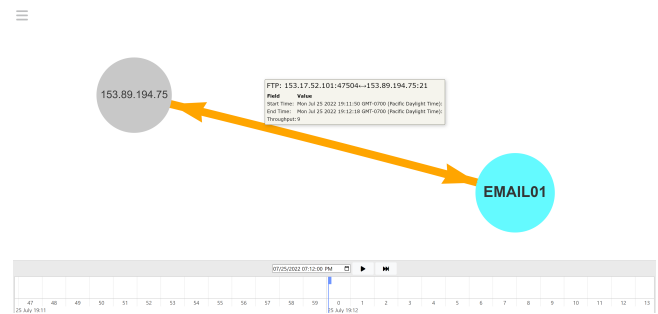
Figure 8. Data exfiltration in scenario. The initial data exfiltration starts from FILE01 as is pushed through EMAIL01, the attacker’s internal pivot point, and out to the malicious remote host, 153.89.194.75.
