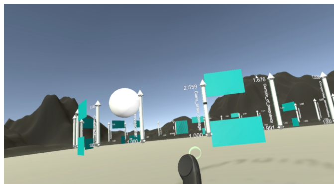
Fig. 4: Lazy Susan menu implemented for the study. Participants spin the menu by rotating their thumb on the controller touchpad.
