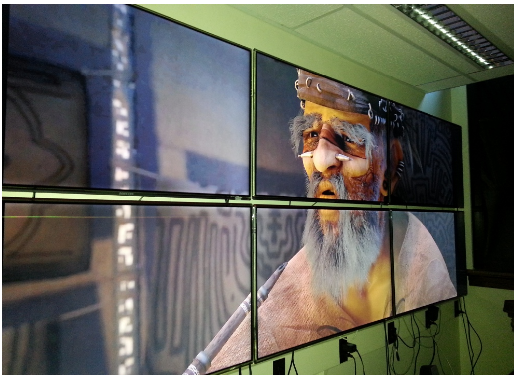
Figure 3: Shard running on a 3 \times 2 tiled LCD display wall where each column of displays is driven by a separate computer. Image credits from the Creative Commons movie Sintel.
