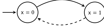
Fig. 17. Illustration of transition system in \iota_x . The dashed line is the private transition.
