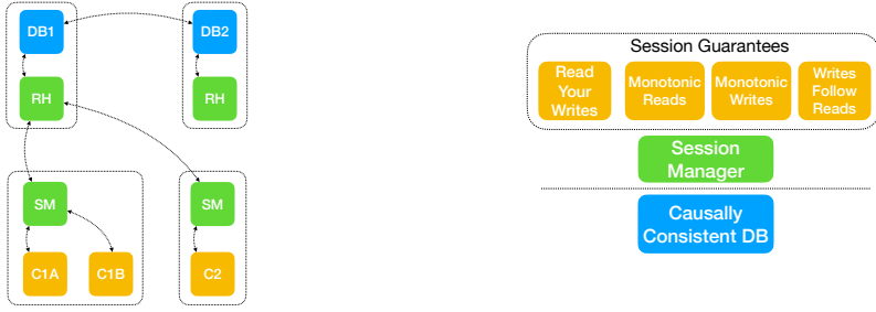
Fig. 10. Clients using the distributed database via the session manager library. Fig. 11. Vertical compositionality of specifications.
