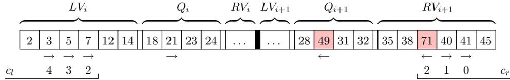
**Figure 8.3:** A verification step for  $\delta = 3$ , with  $k = 1$  initially. The search key is 45. The verification algorithm stops with  $c_r = 0$ , reporting failure. The emphasized elements are corrupted.
