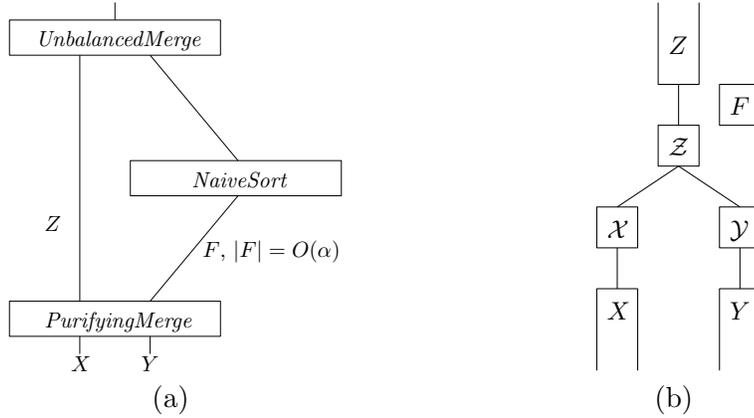
**Figure 6.1:** (a) The structure of the resilient merging algorithm. The input sequences are merged by the *PurifyingMerge* algorithm which creates a  $O(\alpha)$  sized fail buffer which is then merged into the output sequence by the *UnbalancedMerge* algorithm. (b) Overview of the various buffers used in the *PurifyingMerge* algorithm.
