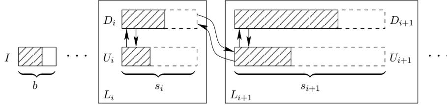
**Figure 7.1:** The structure of the priority queue. The buffers are stored in a doubly linked list using reliably stored pointers. Additionally, the size of each buffer is stored reliably.
