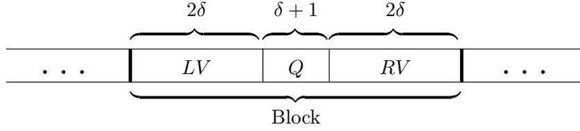
**Figure 8.1:** The structure of a block. The left and right verification segments,  $LV$  and  $RV$ , contain  $2\delta$  elements each, and the query segment  $Q$  contains  $\delta + 1$  elements.
