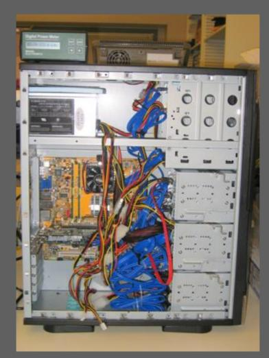
Intel Core 2 Duo T7600 (Mobile CPU) 2 cores, 2 threads, 1.66 GHz 2 GB 2 PCI-e Disk Controllers (8+4 SATA) 1 SATA (onboard) 13 x Hitachi Travelstar 5K160 160 GB Notebook HDD Linux XFS on Linux Software Raid (Striping) NSort (commercial sorter) 59 W 100 W **Power** 2007 JouleSort Winner 10 GB, 100 GB
