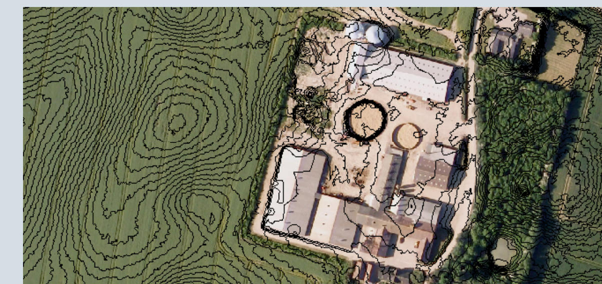
Contour line visualization of a grid. There are obvious flaws in the vicinity of buildings (where no input points are available)
