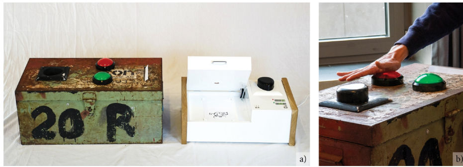
Figure C.1: a) The two components of the Machine Learning Machine; the Trainer (left) and the Evaluator (right). b) A user labelling a drawing using the Trainer to train a machine learning model.
