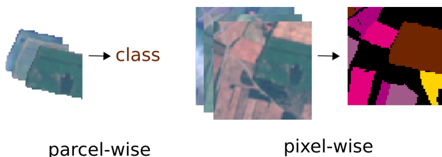
Figure 3.1: Crop classification of SITS with deep learning is either performed parcel-wise, which requires knowledge of the parcel borders, or pixel-wise, which does not. For the latter, we show here a semantic segmentation approach, where a satellite image time series is mapped to a segmentation image containing pixel-wise predictions.
