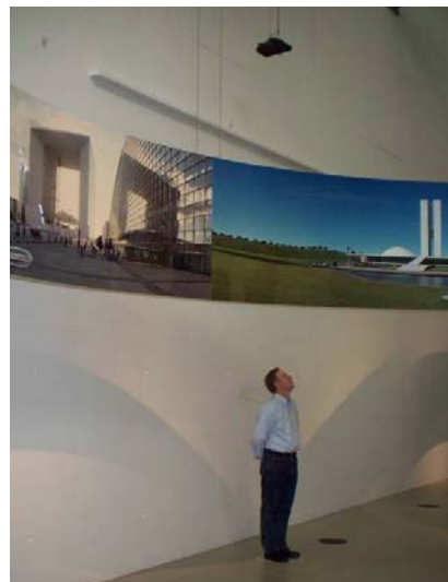
Figure 2: A directional speaker above an audio spot marked by a silver circle on the floor.
