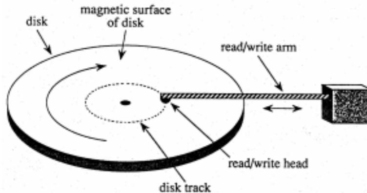
Fig. 2. Platter of a magnetic disk drive.
