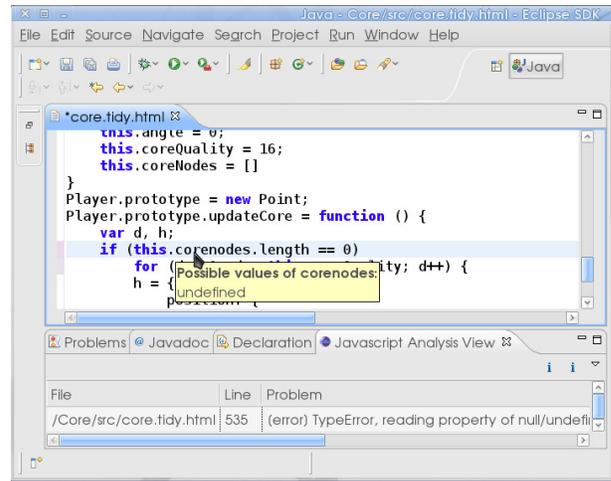
Figure 4: The TAJIS analysis plug-in for Eclipse, reporting a programming error and highlighting the type inferred for the selected expression.
