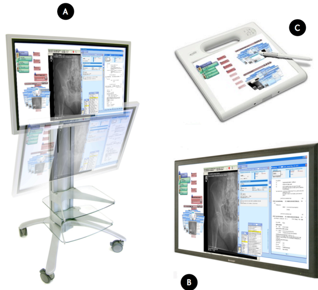
Figure 3.19 The interaction is distributed on three types of displays. (A) is a mobile LCD, (B) is a fixed LCD, and (C) is a mobile personal device
