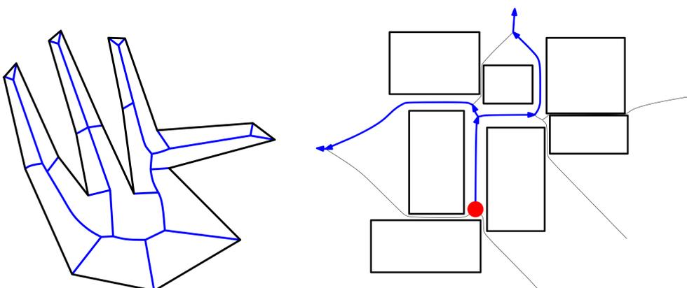
The order-k Voronoi diagram of line segments appears in the geometric min-cut problem that can model, among others, the VLSI critical area extraction problem.
